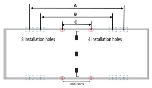
$\diamond$  Use mounting holes of A or B or C , safety factor  $\gamma_{m=1,5,m}$  and this value can decrease if modules are not mounted following the instructions above.
